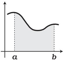
$$\int_a^b p(x) dx \approx \sum_{x=x_0, x_1, \dots, x_n} p(x)\Delta x$$
